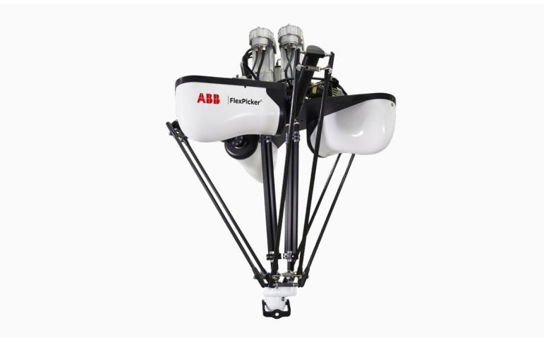
IRB 365 FlexPicker® five axis Delta robot fastest for lightweight product picking
